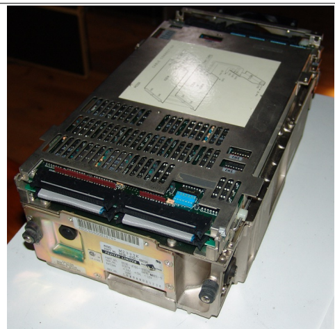
Gould model 8887 (Fujitsu M2333K) 8" SMD disk, size 340MB
